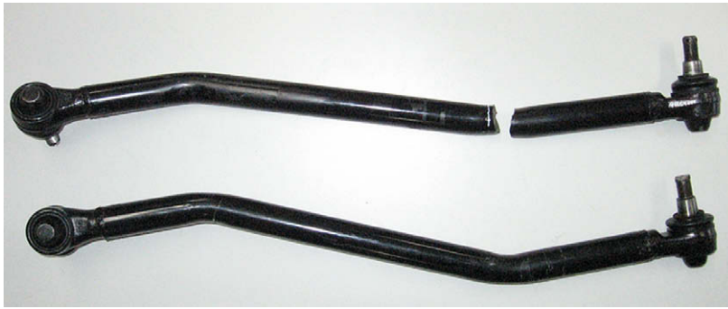
Fig. 1. Link assembly in steering system.
