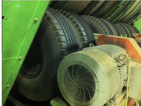
Fig. 2. System of rubber tyres for actuation of cylindrical drum shell.
