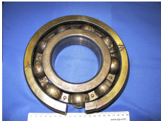
Fig. 1. The failed DE bearing covering with the brown deposit.
