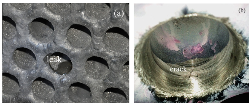
Fig. 1. Leakage position and crack appearance on the tube of the water-gas waste heat boiler. (a) leakage position and (b) crack appearance.
