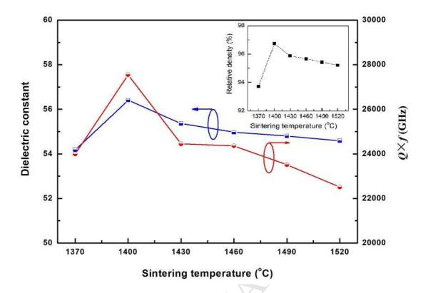
$0.5Ca_{0.6}La_{0.267}TiO_3$ - $0.5Ca(Mg_{1/3}Nb_{2/3})O_3$  ceramics were successfully prepared by a reaction-sintering process. Fine microwave dielectric properties of  $\epsilon_r$  = 56.4,  $Q\times f$  = 48550 GHz and  $\tau_f$  = +8.7 ppm/°C for 5CLT-5CMN ceramics with high density sintered at 1400 °C for 4 h were obtained.
