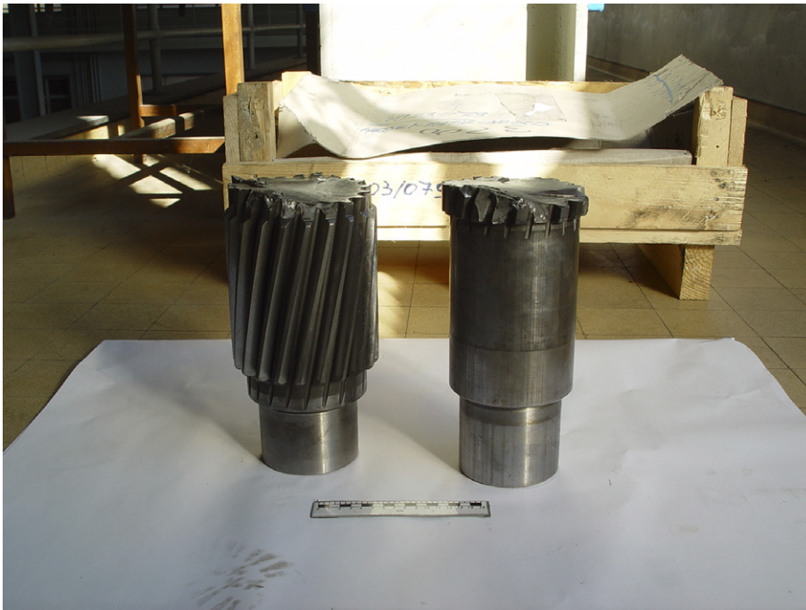
Fig. 1. View of the two parts of the failed axle.
