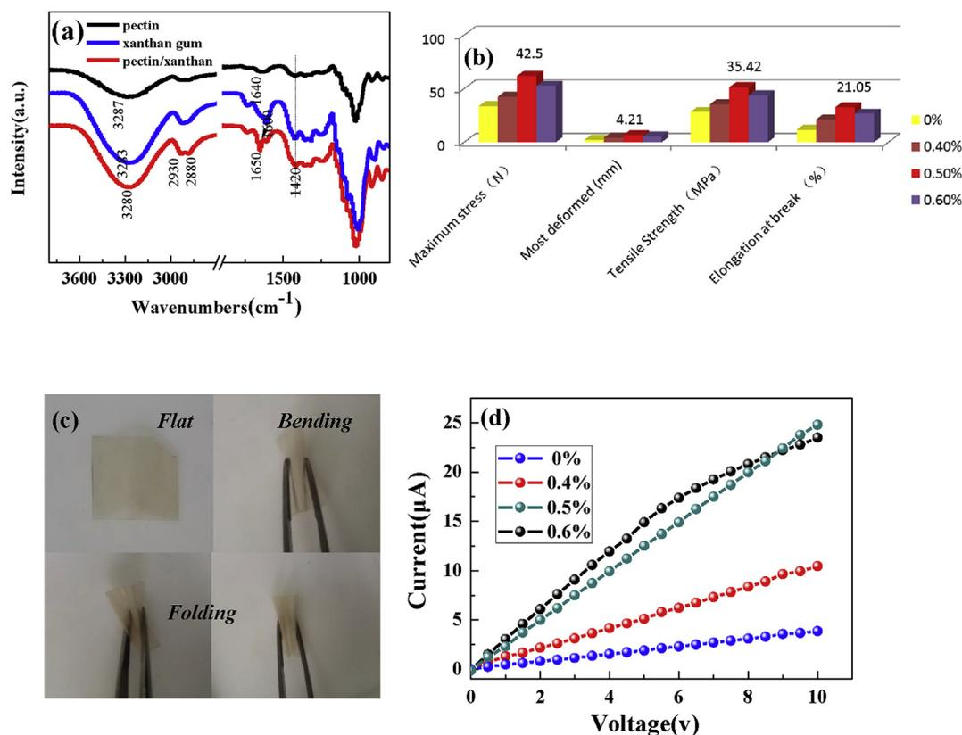
**Fig. 1.** a) FT-IR spectrogram of pectin, xanthan gum and blend film. b) The mechanical properties (including tensile strength, elongation at break, etc.) of the xanthan gum blend films at different concentrations (0%, 0.4%, 0.5% and 0.6% w/v). c) The physical behaviors of the blend film in different states. d) The typical current-voltage characteristics of the xanthan gum blend films at different concentrations.
