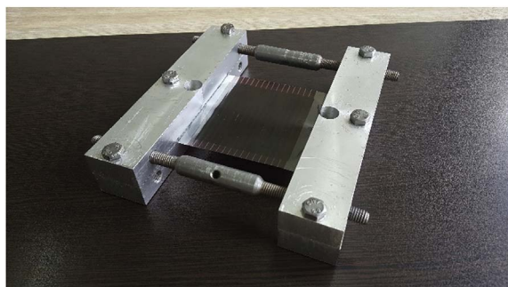
Fig. 2. The test structure used for straining the solar cells.
