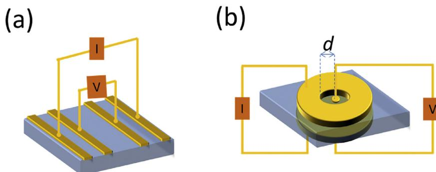
Fig. 1. Schematic of the (a) in-plane and (b) through-plane four-probe electrical conductivity measurement setup.
