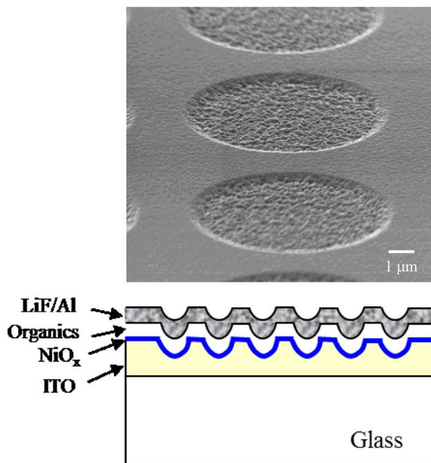
Fig. 1. Schematic of OLED device structure with a  $\text{NiO}_x$ /recessed ITO anode and the SEM image of a 150 nm recessed ITO film.
