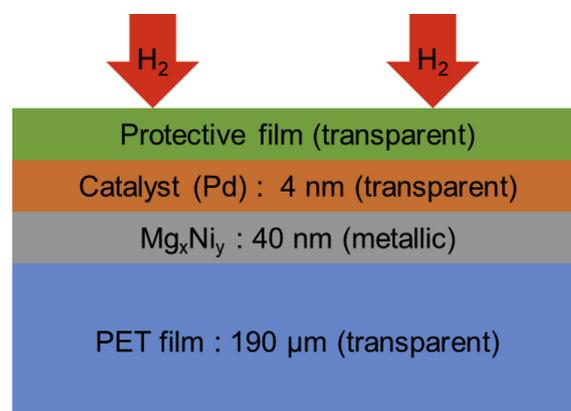
Fig. 1 – Schematic of a HSAF [33].
