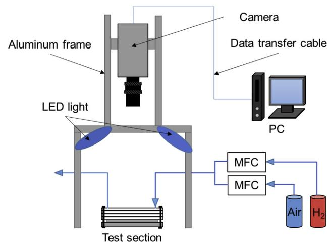
Fig. 2 – Overall view of the visualization apparatus.
