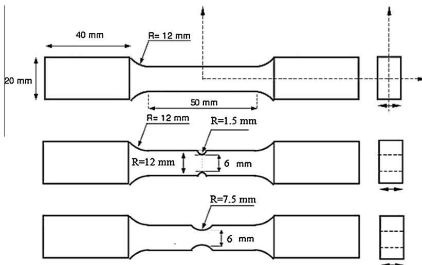
Fig. 1. Geometry of the tensile testing specimens.
