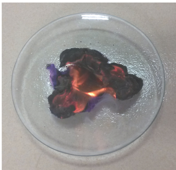
Fig. 1 – Combustion process of the absorbent cotton impregnated with cobalt acetate.
