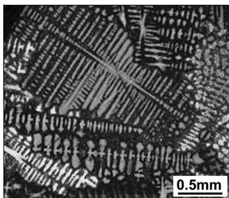
**Fig. 1.** Dendritic structure in transversal section of the specimen gauge length.
