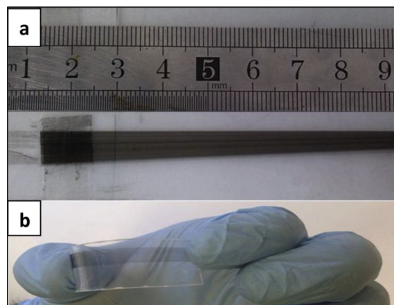
Fig. 2 – (a) Optical image of WMCNTs sheets extracted from vertical arrays and (b) MWCNTs as a sheet over a flexible plastic substrate.
