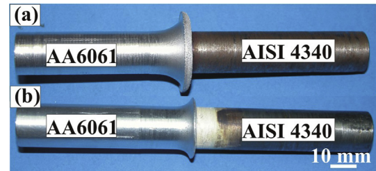
Fig. 1. Macrograph of friction welded AA6061-AISI 4340 (a) without silver interlayer and (b) with silver interlayer.
