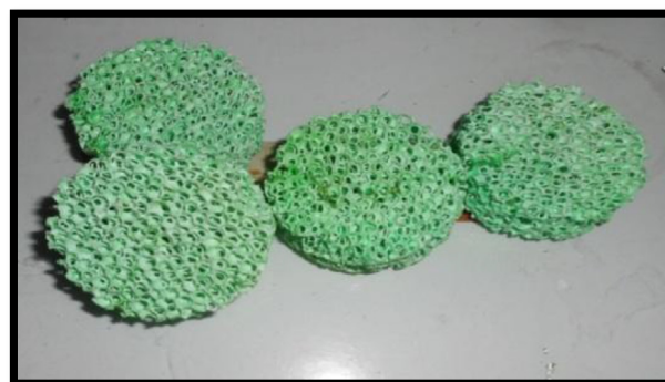
Fig. 1 – Alumina foam type catalyst with Ni coating.
