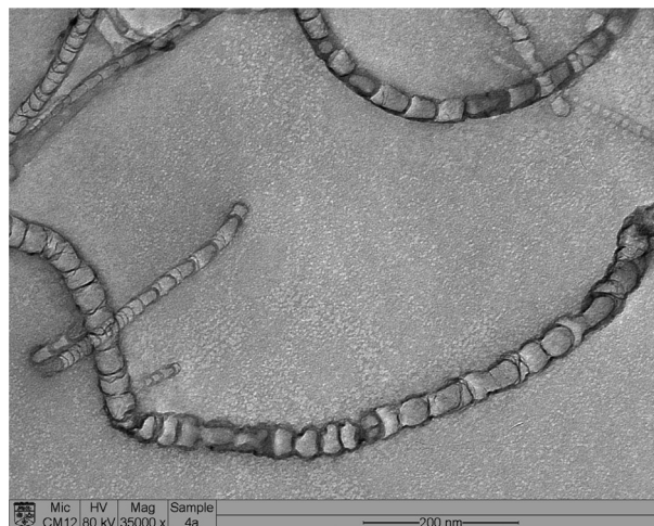
Fig. 1 – TEM image of NCNT at magnification of 35,000 × .
