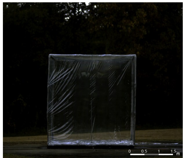
Fig. 1 – A photograph of the experimental rig (27 m 3 cubic plastic tent).
