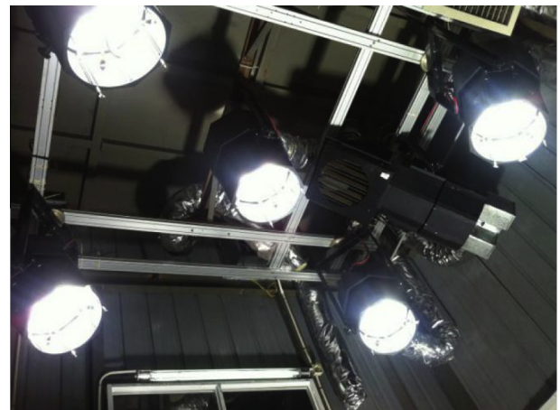
Fig. 1. Solar simulator with five 7 kW Xe-arc lamps.
