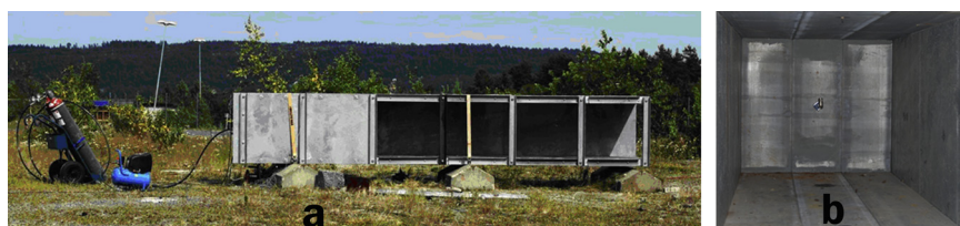
Fig. 1 – Experimental channel at Norward test facility a) 6 m long channel with a side wall made up of 2 m steel wall and a 4 m transparent polycarbonate wall. b) Closed end wall with nozzle in centre pointing upwards.
