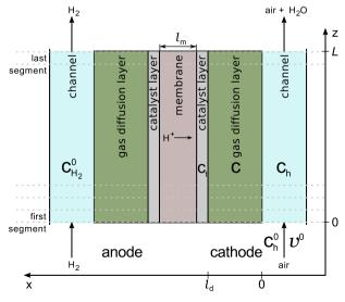
Fig. 1 – Schematic of a fuel cell.
