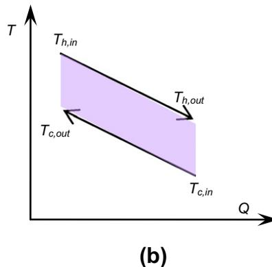
Fig. 1. Heat transfer process in a counter-flow heat exchanger: (a) hot and cold fluids and (b) heat transfer process shown in a  $T$ – $Q$  chart.
