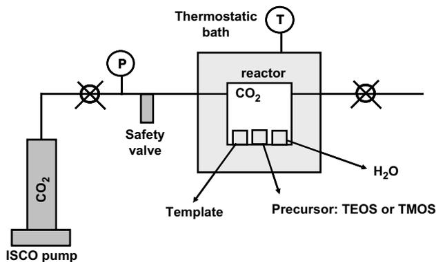
Fig. 1. Experimental set-up used to infuse and react TEOS or TMOS into the 3D-latex array templates.
