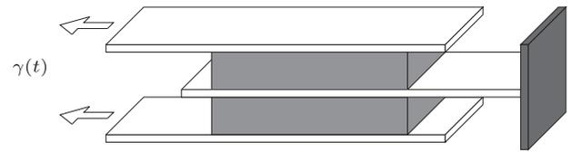
Fig. 1. Double-shearing specimen.
