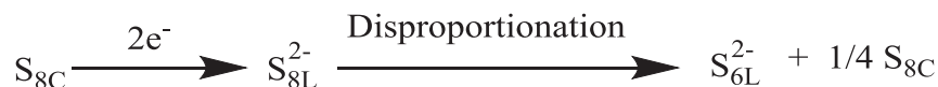
Scheme 1. Proposed mechanism of 2-electron electrochemical reduction process followed by chemical reactions (2EC).
