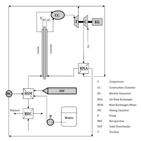
Fig. 1. Schematic representation of integrated DU-SOFC/GT system.
