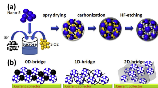
Fig. 1. Schematic of the fabrication of a) porous Si–C composite and b) conducting agents bridged electrodes.
