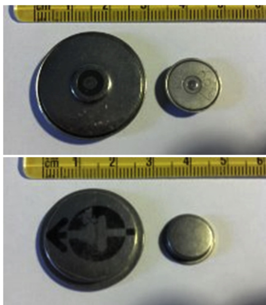
Fig. 1. 25 mAh and 100 mAh Li– \text{TiS}_2 Cells fabricated by Exxon in 1978: (top) top of the cells, and (bottom) bottom of the cells.
