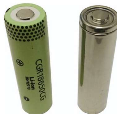
Fig. 1. Panasonic CGR18650CG LIB cell with (left) and without (right) plastic packaging.
