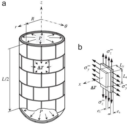
**Fig. 1.** Illustration of the studied configurations. (a) Lower-half part of cryogenic tank recovered with foam panels and subjected to internal pressure  $P$  and temperature drop  $\Delta T$ ; (b) plane geometry approximation of an elementary unit.
