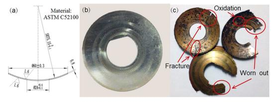
Fig. 2. The thrust washers in the differential. (a) A schematic technical drawing. (b) A photograph. (c) Failure of thrust washer.
