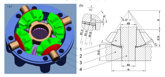
Fig. 1. The model of the differential (a) The 3D model of the differential (b) The schematic technical drawing of the spider gear-thrust washer-case assembly and 1 — spider gear, 2 — thrust washer, 3 — differential case, 4 — pinion shaft.
