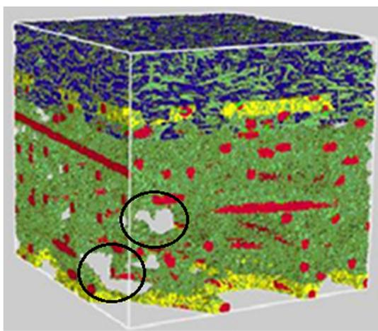
**Fig. 1.** 3-D rendering of GDL structure with carbon fiber in red, fill matrix in green, PTFE loading in yellow, MPL structure in blue, and some large pores circled. Made with GeoDict<sup>®</sup> software, and provided by Ballard Power Systems. (For interpretation of the references to color in this figure legend, the reader is referred to the web version of this article.)
