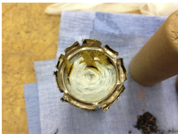
Fig. 1. Top view cutout of a typical Li-ion cylindrical cell.
