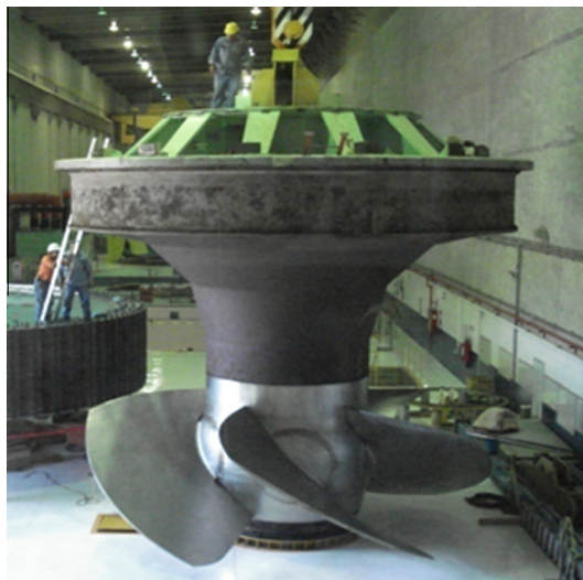
Fig. 1. Kaplan turbine runner.
