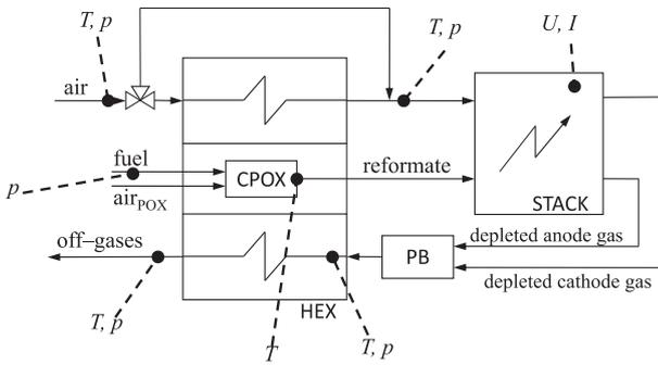
Fig. 1. Schematic flow diagram of the HoTbox™. Reproduced from Ref. [11] by permission from Wiley.
