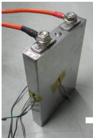
(a) Temperature measuring point
