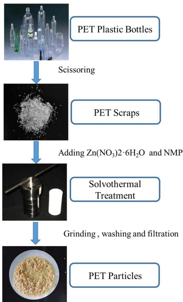
Scheme 1. The process to produce active PET particles.
