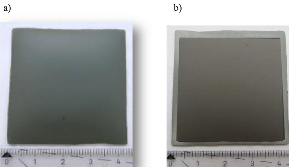
**Fig. 1.** a) Picture of an intermediate 4.5 \* 4.5 cm<sup>2</sup> size NiO–BCZY8/BCZY8–ZnO half-cell co-fired and b) the same PCC after printed BSCF–BCZY8–BSCF air electrode.
