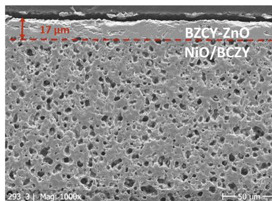
**Fig. 2.** Scanning microscopy cross-section of a 20 cm<sup>2</sup> size NiO–BCZY8/BCZY8–ZnO half-cell.
