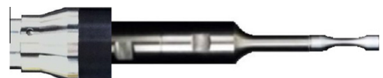
Fig. 3. Photograph of the structural body of the ultrasonic fatigue tester (UFT-20X, MediSource-Plus corp).
