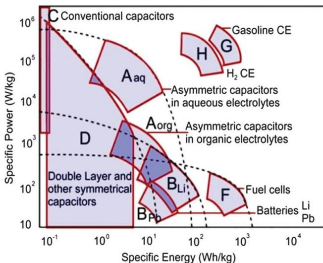
Fig. 1. Ragone plot with specific energy and power for a diverse range of energy storage devices [6].
