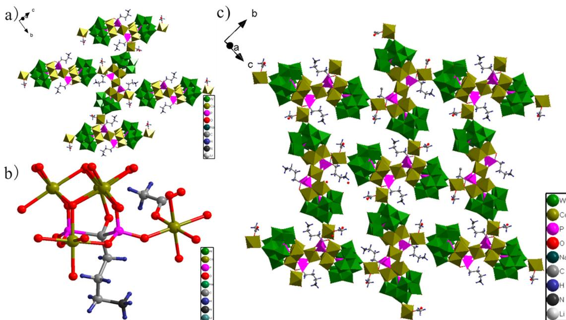
Fig. 2. (a) Linking modes between the sandwich polyoxoanions and the linking units  $\{Co(H_2O)_3(CH_3COO)\}$ ; (b) coordination modes of Ale ligands and the central  $\{Co_7\}$  cluster; (c) 2D spatial configuration of **1**.
