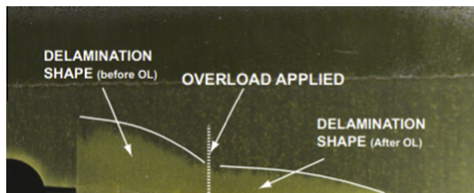
Fig. 2. Kink phenomenon in the delamination shape caused by overload [16].
