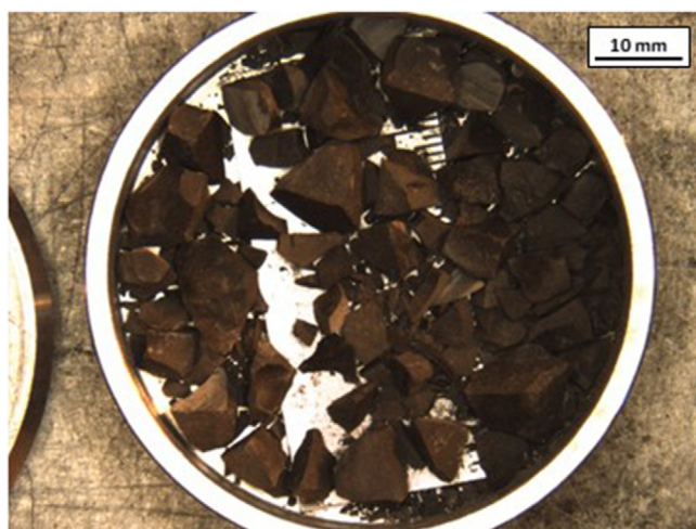
Fig. 1. Irradiated thoria fuel removed from sheath.
