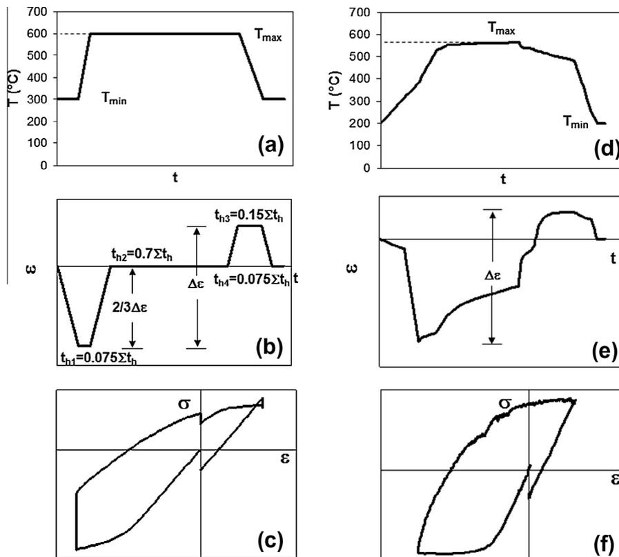
Fig. 2. Single-stage service-type [9] temperature cycle (a), strain cycle (b), corresponding hysteresis loop (c), service-like [10,11] temperature cycle (d), strain cycle (e) and corresponding hysteresis loop (f), both representing cold start cycle, sum of hold times  $\sum t_h = t_{h1} + t_{h2} + t_{h3} + t_{h4}$ . For more details refer to [6,8,9,13].
