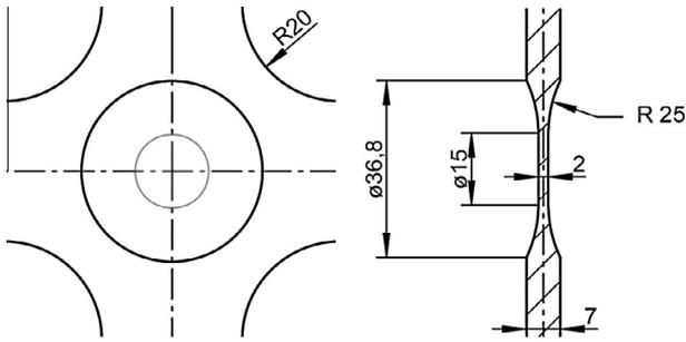
Fig. 1. Cruciform specimen used for biaxial creep fatigue experiments.
