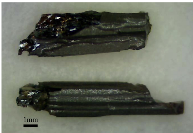
Fig. 2. Single crystals of \alpha\text{-Li}_3\text{Fe}_2(\text{PO}_4)_3 obtained by a flux method.
