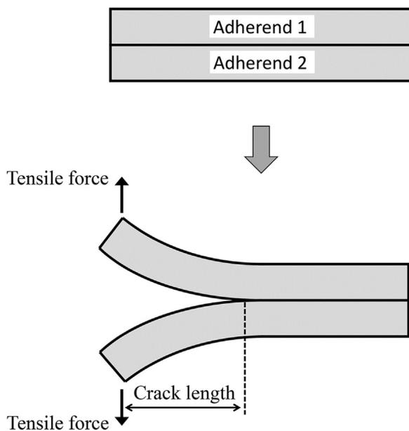
Fig. 1. DCB test that determines the mode I critical energy release rate.
