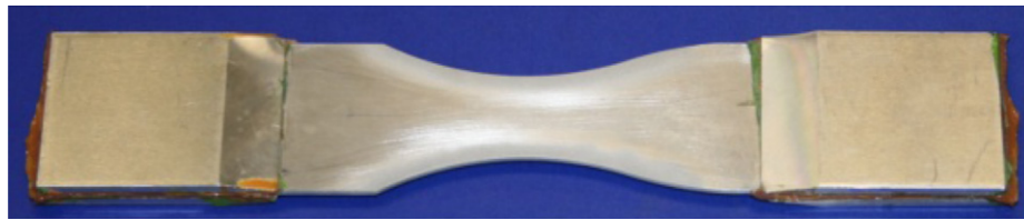
Fig. 2. Aluminium alloy 7075-T6 dog-bone specimen with edges treated with the Australian grit-blast silane surface preparation procedure.
