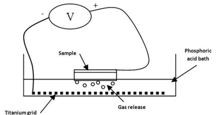
Fig. 1. Schematic representation of set-up for phosphoric acid anodisation (PAA).
