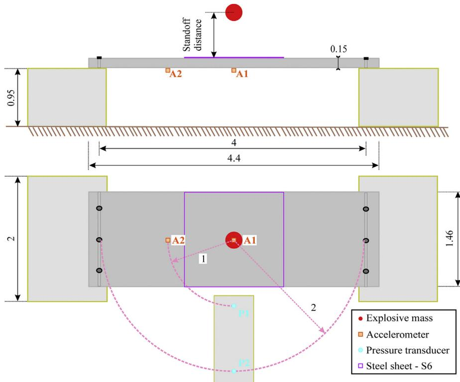
Fig. 1. General blast test set-up. Measurement devices locations in slabs S1, S2 and S3, and steel sheet used in slab S6 (units: m).
